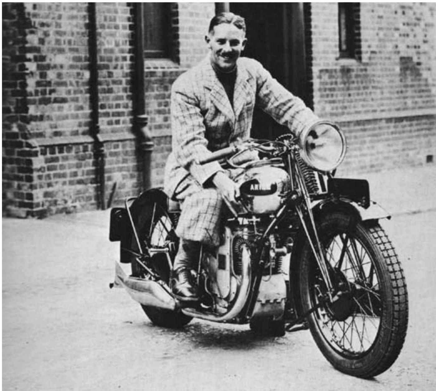
The Ariel Square Four, as first manufactured, employed an overhead camshaft. This is the 1932 600cc OHC model, new features of which embraced a redesigned cylinder head, and an instrument panel insert on the fuel tank's top face.
